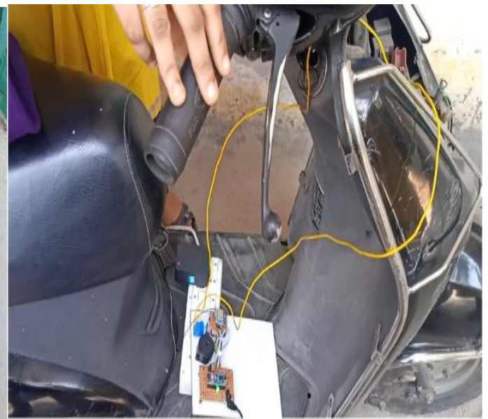
Fig 6. Transmitter setup fixed in vehicle
